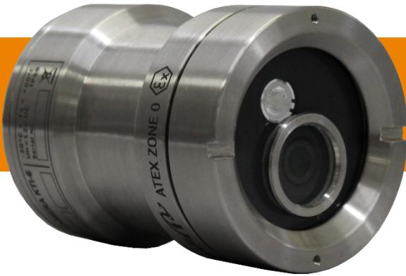
The intrinsically safe camera KTi-7 is used to transmit real-time images from methane/coal dust explosion hazard areas - group I and areas classified as zones 0, 1, 2 (G) or 20, 21, 22 (D) - group II.
